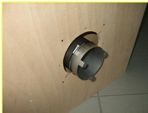
3.) Push the mixing tube together with the hose clamp into the hole from the rear.
