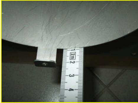
6.) Adjust the front flange plate. Very important is that the lower end of the mixing tube is around 2mm closer to the flange plate than the upper end of the mixing tube. This is the best way to guarantee that the FogMaker is tilted to the front and the condense water can flow out.
