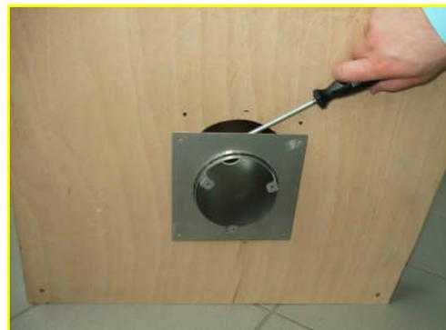
7.) Adjust the upper edge of the mixing tube to the flange plate.
